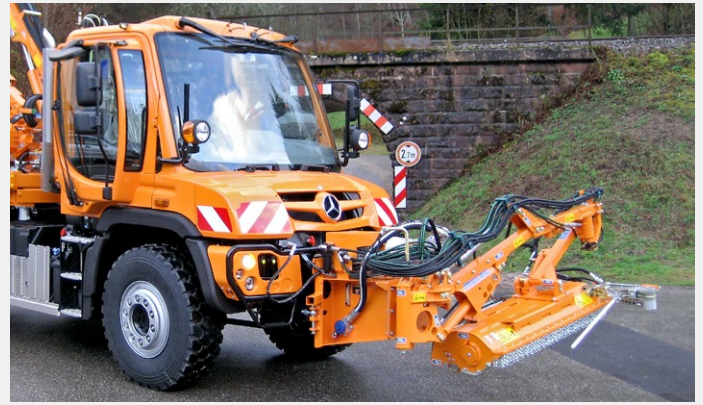
Verge mower MRM 300 in transport position
