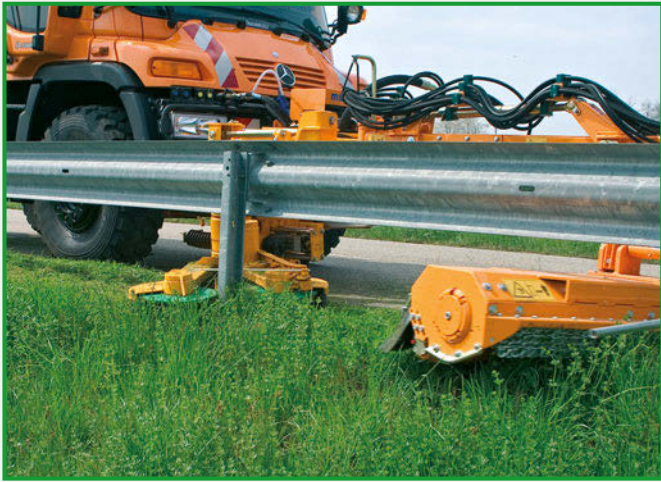
Suitable for mowing beneath crash barriers
