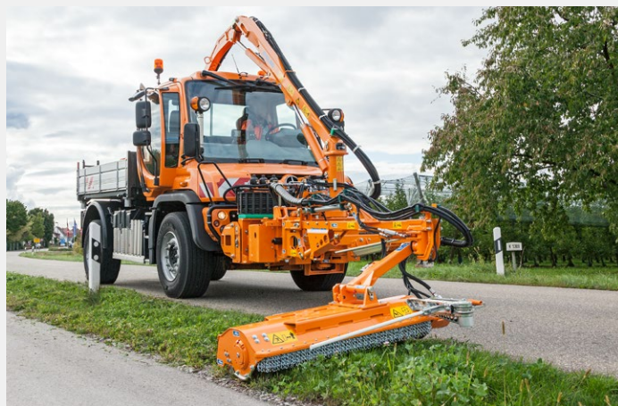
Solo operation of the verge mower
