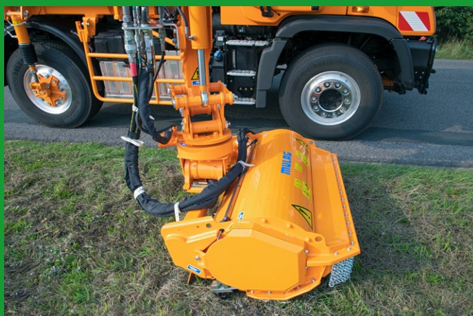
Tilt/swivel device for swiveling and tilting the working attachment
