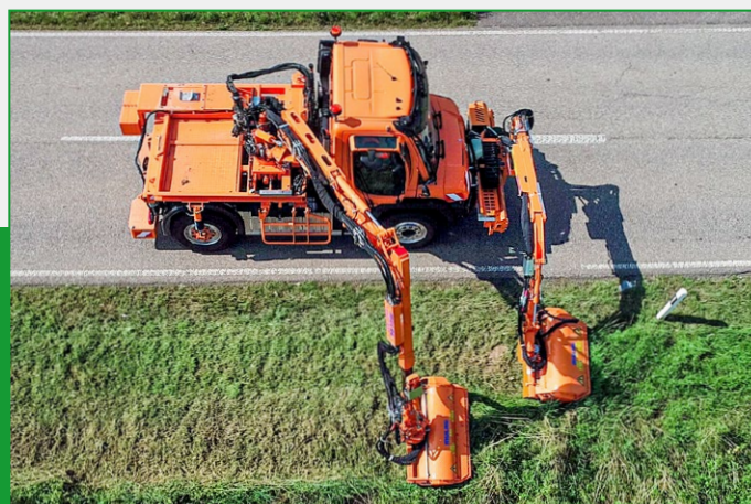
Combination operation - both mowing heads in the operator's field of vision
