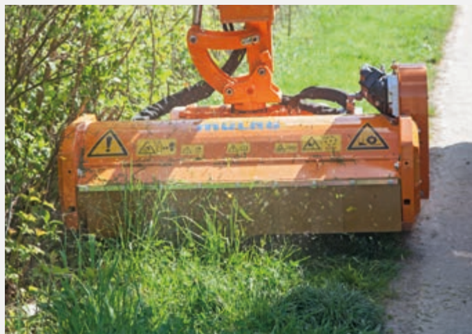
GMK 1200 with closed protection for use in grass
