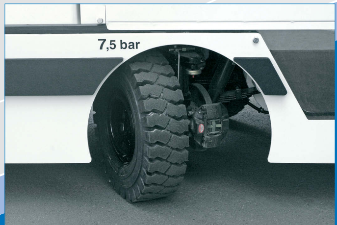
Optimized steering geometry up to 70° with low tire attrition
